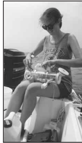
Erin uses a Van Dorn water sampler that allows samples to be taken from below the water's surface.
